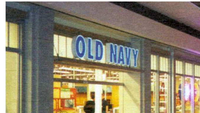
unacceptable - letters exceed 16" high
