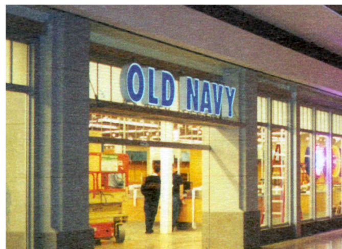
unacceptable - letters exceed 16" high
